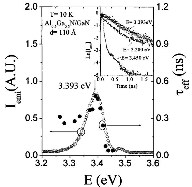
FIG. 5. Emission energy dependence of the decay lifetime of the 2DEG emission line measured at 10 K. The time-integrated emission spectrum is also shown. The inset shows the temporal responses of the PL emission measured at several different emission energies.
