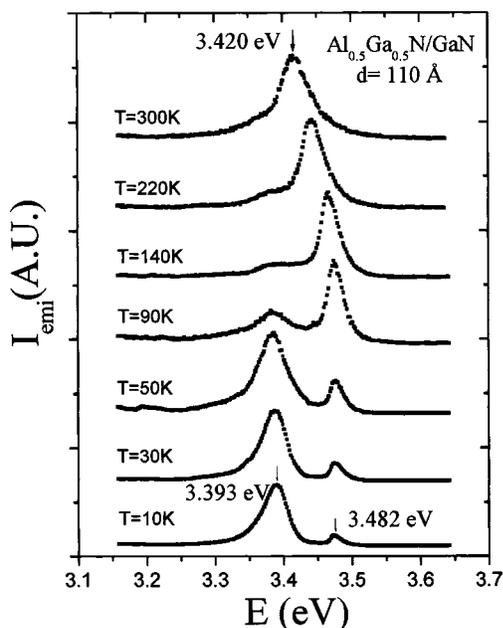
FIG. 2. PL spectra of a representative  $\text{Al}_{0.5}\text{Ga}_{0.5}\text{N}/\text{GaN}$  heterostructure with  $d=110 \text{ \AA}$  (KSU A-166) measured from 10 to 300 K.
