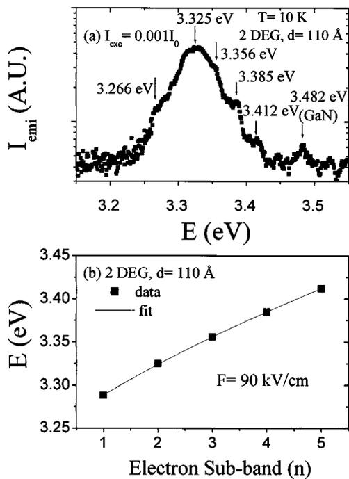
FIG. 4. (a) Low-temperature (10 K) PL spectrum of an  $\text{Al}_{0.5}\text{Ga}_{0.5}\text{N}/\text{GaN}$  heterostructure under low excitation intensity ( $10 \text{ W}/\text{cm}^2$ ) and five emission peaks are resolved. (b) The least squares fit (solid line) of the observed five emission peak positions (solid squares) with Eq. (1).
