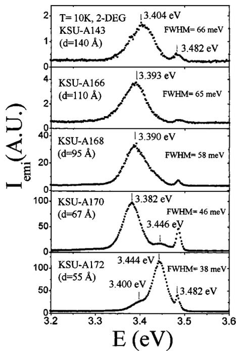
FIG. 1. Low-temperature (10 K) cw PL spectra of  $\text{Al}_{0.5}\text{Ga}_{0.5}\text{N}/\text{GaN}$  heterostructures with different top AlGaN layer thicknesses ( $d$ ).
